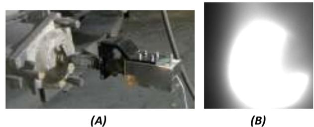
**Fig 3: (A) Mechanical Arrangement for Tuyere Monitoring System (B) The live image of Tuyere through the Peephole**
